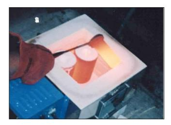
After the investment has setup, it has to be fired to remove the wax, by burning the wax out. The mold is slowly heated to about 450 degrees for the burn out. Once the wax is burned out, leaving the voids that the bronze will fill up. The mold is then heated up to around 1200 degrees, so the mold does not chill the bronze as it is being poured.
