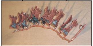
The sprues have to be cut off, and then the exposed areas are filed down, and matched with the rest of the piece. The towers are given a rough polishing, and then given a patina. Patinas can either be artificial, like liver of sulfur, or more natural, with exposure.
